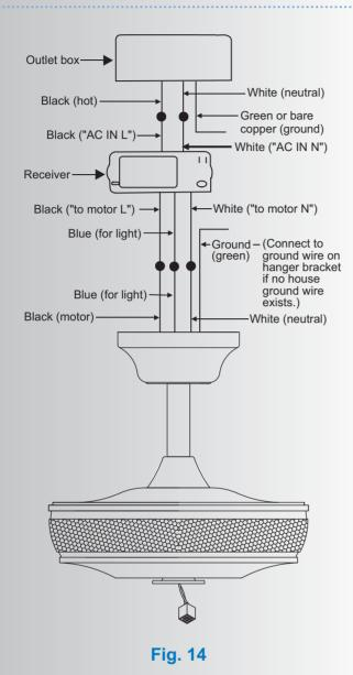
Step 2. Motor to Receiver Electrical Connections: (Fig. 14)
